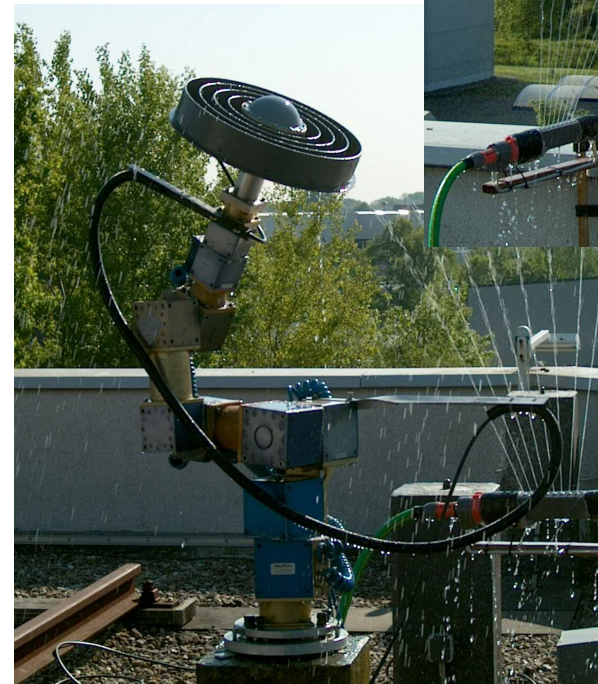
Sprinkling of ASH700936D_M NONE during antenna calibration
