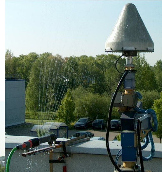
Sprinkling of ASH700936D_M SNOW during antenna calibration
