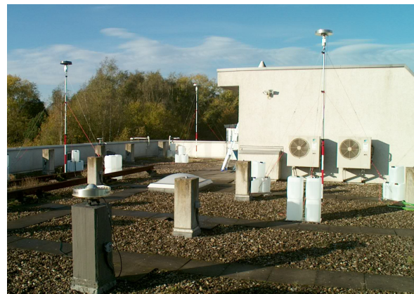
Fig. 2: Near-field free stations on poles and GNSS reference stations (on pillar in front, on roof partly obstructed)
