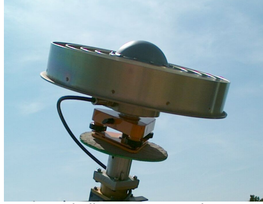
Fig. 5: round pillar reconstruction with a Dorne Margolin choke ring antenna on the robot, diameter 20 cm
