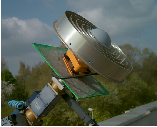
Fig. 6: quadratic pillar reconstruction with a Dorne Margolin choke ring antenna on the robot, edges 30 cm
