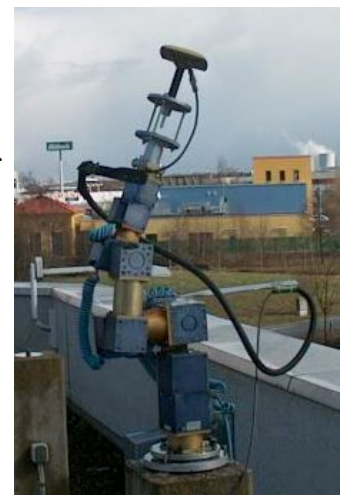
Fig. 1: near-field calibration of a TPSPG_A1 antenna on a special mount/mast
