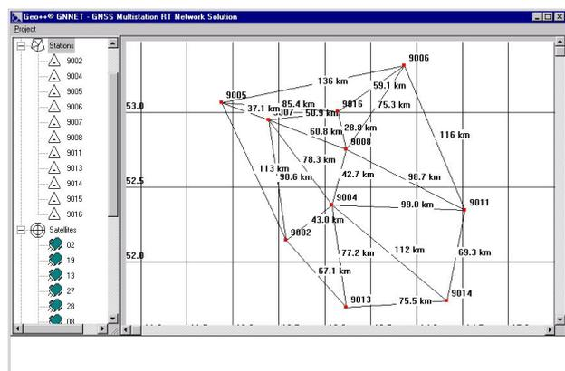
Fig. 8 : Screen shot of reference station distribution of GNET, main module of GNSMART, Brandenburg RTK network, Germany
