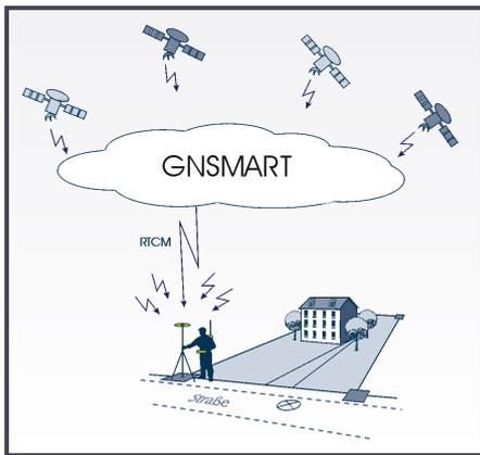
Fig. 1: Millimeter Precision for a GNSS rover with ultimate correction data provided by GNSMART
