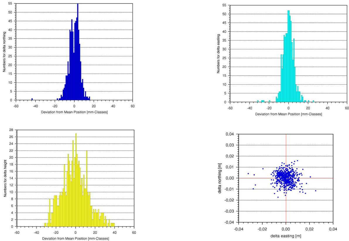
Fig. 4 : Histogram of deviation from the mean position in northing, easting, height (millimeter classes) and horizontal position plot (units are meter), GSI RTK network, Japan
