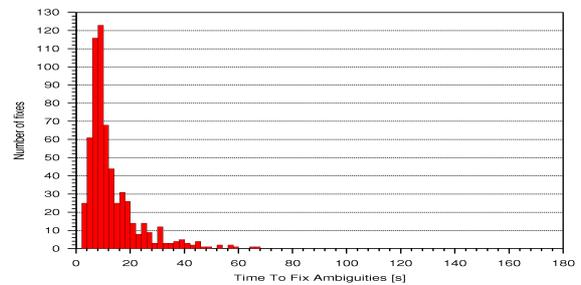
Fig. 6 : Histogram of Time to Fix Ambiguity (TTFA): mean is 14 seconds, GSI RTK network, Japan
