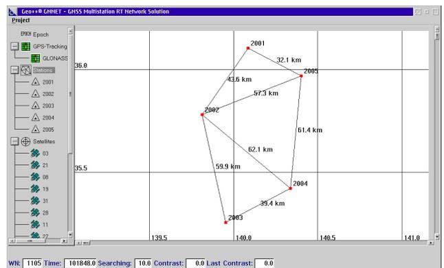
Fig. 3: Screen shot of reference station distribution of GNNET, main module of GNSMART, GSI RTK network, Japan
