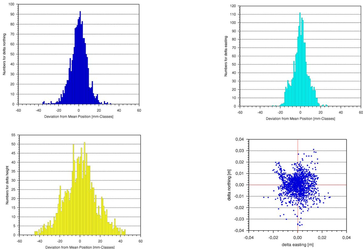
Fig. 7 : Histogram of deviation from known position in northing, easting, height (millimeter classes) and horizontal position plot (units are meter), Brandenburg RTK network, Germany
