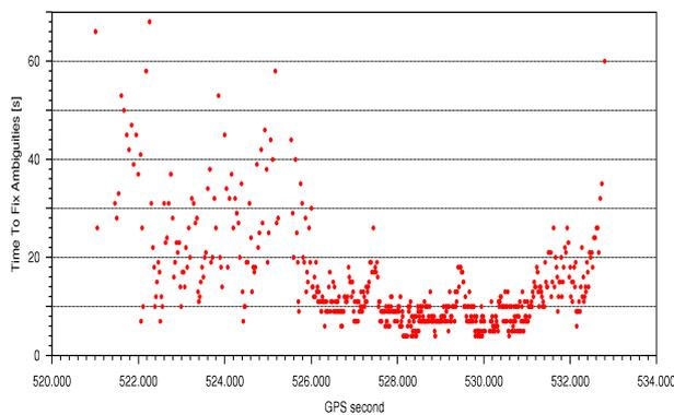
Fig. 5 : Time to Fix Ambiguity (TTFA): mean is 14 seconds, GSI RTK network, Japan
