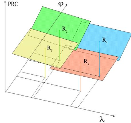
Fig. 2: Linear FKP planes for four reference stations
