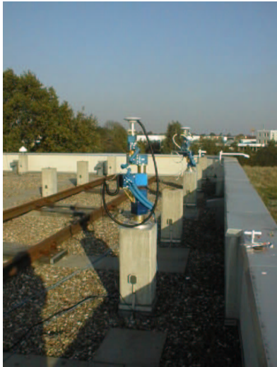
verification of Absolute Multipath Calibration using two robots and one antenna/site to be MP calibrated
