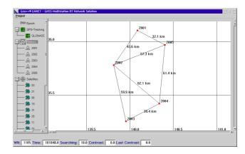
Fig. 3: Screen shot of reference station distribution of GNNET, main module of GNSMART
