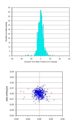
Fig. 4: Histogram of deviation from the mean position in northing, easting, height (millimeter classes) and horizontal position plot (units are meter)
