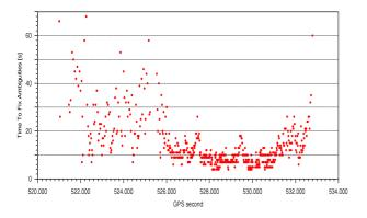
Fig. 5: Time to Fix Ambiguity (TTFA): mean is 14 seconds
