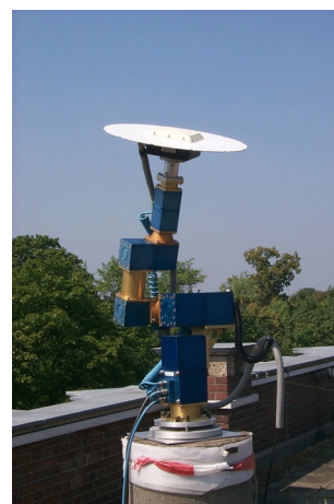
Fig. 1: Absolute field calibration of PCV with a robot.
