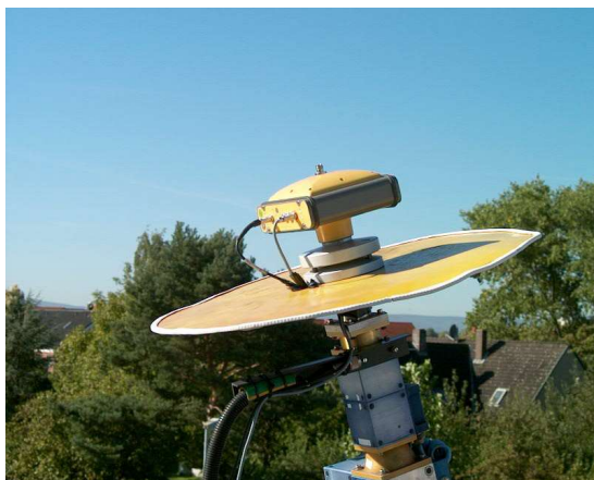
Fig. 1: Absolute robot calibration of a TPSHIPER_PLUS mounted on a round car roof cut-out
