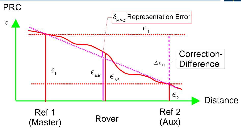
Rover receives Raw Data of the Master Station and Correctiondifferences for the Aux-Stations (min. 2)
